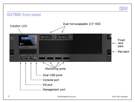
In this diagram, you see the front panel of the GX7800 appliance. You can use the 5-button LCD for initial network configuration, for restarting or shutting down the appliance, and for obtaining IPS version information. You can also use it to view the serial number of the appliance.
