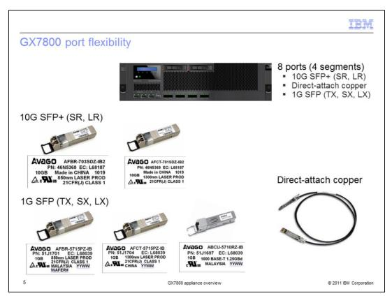
The GX7800 has port flexibility. The small form-factor pluggable (SFP) transceivers that work with the appliance are listed on the slide. The short range (SR) and long range (LR) transceivers support 10 Gb segments.
