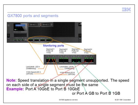
Speed translation within a segment is not supported. As you can see from the example on the slide, the ports within a segment must be set at the same speed. You cannot have a 10 Gb router plugged into port A and a 1 Gb switch plugged into the paired port B.
