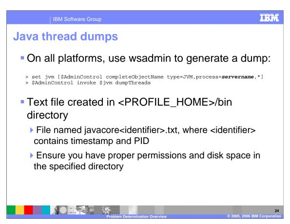
The wsadmin command shown here is particularly useful on Windows®, because you cannot generate a dump by sending a signal to an arbitrary process, as you can under Unix®.
