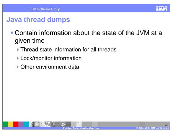
Thread dumps are snapshots of the state of the JVM at a given time. They show what every thread was doing at the time of the dump, and the state of monitors, and other information about the JVM.
