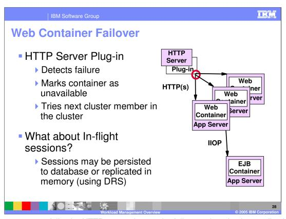
If a server process fails, the HTTP server detects the failure and marks that application server as unavailable. It then routes the request to the next cluster member.
