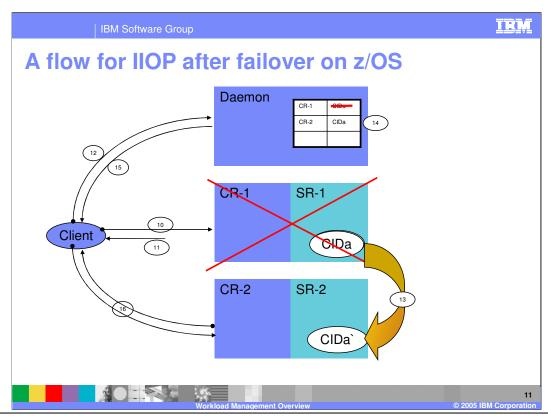
This graphic shows what happens when an object is no longer available. Here we have shown a complete server stopping and the client then sending a request to the object. Again there are several scenarios that might require an object to be moved, but this case demonstrates the key points. Following the numbered arrows as before we have:
