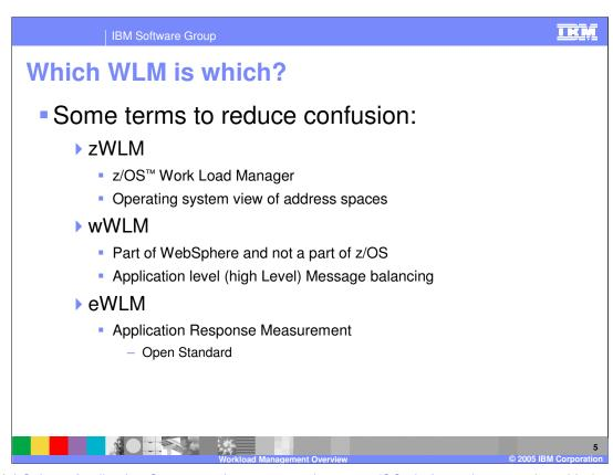
With WebSphere Application Server version 6.0.1 running on a z/OS platform, there are three kinds of Work Load Managers active. These three Work Load Managers cooperate to make WebSphere perform optimally.
