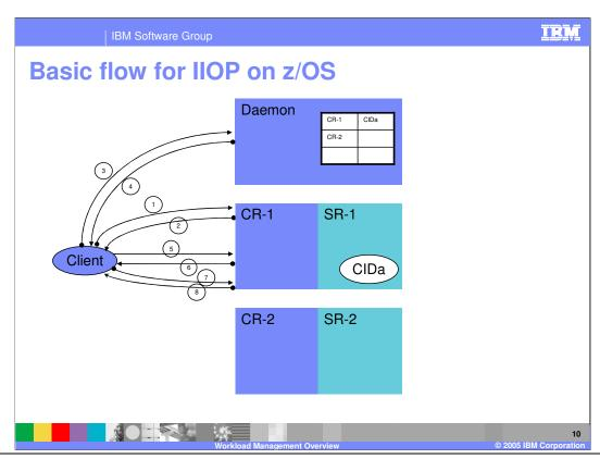
This graphic shows the a basic flow of an IIOP location request on z/OS and though there are many possible scenarios, this one demonstrates the key points. The client shown can be any object invoking an EJB bean, such as another application server or an edge server. The arrows represent an ordered sequence of events.
