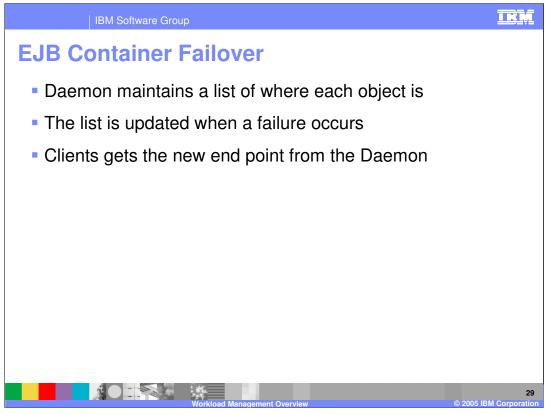
On z/OS platforms, EJB container failover is still handled by the daemon. The system detects a failed server and moves the internal pointers to a new copy of the object on a different server. When an EJB client detects the failure, a locate request is sent to the daemon which returns the new object.
