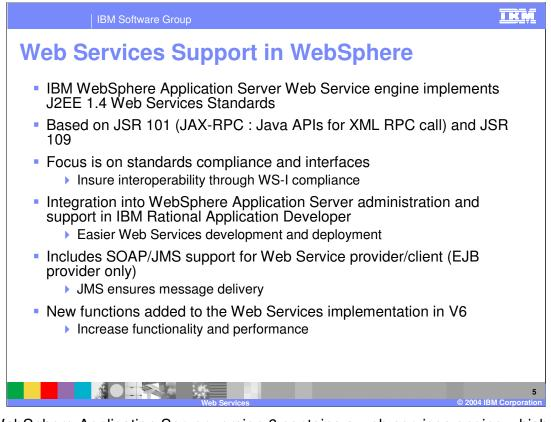
The WebSphere Application Server version 6 contains a web services engine which supports the J2EE 1.4 standards for applications. The web services engine was designed to support both JSR 101, or JAX-RPC and JSR 109, or J2EE web services. These specifications were covered in greater detail in the Web Services overview lecture. By adhering so closely to these standards, the web services engine focuses on interoperability and providing interfaces to internal functions in the runtime.
