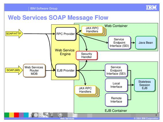
This slide shows how a SOAP message being sent to a Web Service, enters the J2EE runtime that's part of the Application Server. There are two separate flows here, depending on the transport protocol for the SOAP message, either HTTP or JMS. WebSphere Application Server version 6 supports both.
