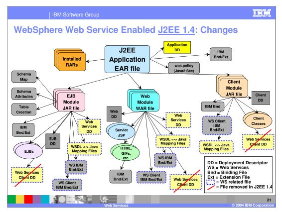
This slide is a visual example of the deployment descriptor changes. Showing the removal of the Web Services client.xml file. The rest of the files associated with Web Services have not been changed.
