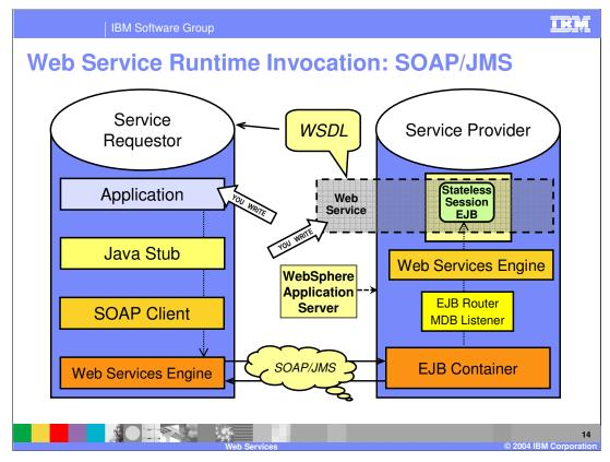
This slide shows the differences in a call to a Web Service using JMS. The primary difference is that instead of using an HTTP client to send the message, a JMS client is used. And on the provider side, the message is received by a message driven bean running within the EJB container, rather than by a servlet running within the Web container.
