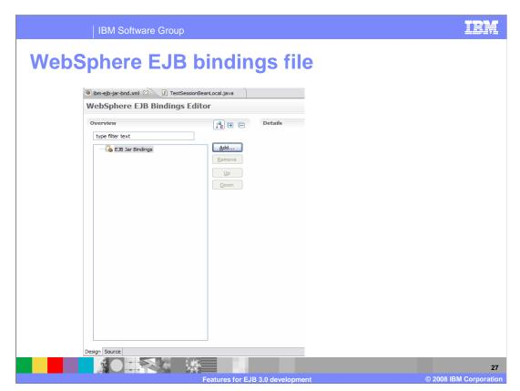
Shown here is a screen capture of the EJB bindings file editor that is opened when the bindings file is generated.
