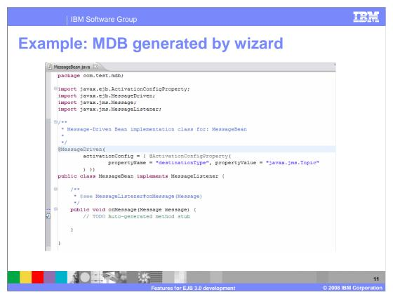
Shown here is a screen capture of generated message driven bean code. You can see that the at message driven annotation is added to the top of the class definition. Annotations are added to specify the destination type, in this case you can see that the destination type is a topic.
