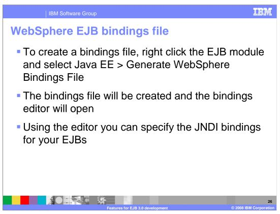
A bindings file can be generated similar to creating an EJB deployment descriptor. You can do this by right clicking on the EJB project and selecting the Java EE submenu; followed by clicking the menu option to generate WebSphere bindings file.
