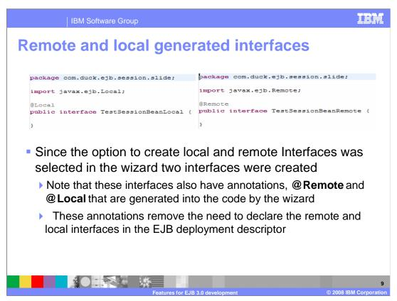
The option in this case for local and remote interfaces was selected, so the interfaces have also been generated in the EJB project.
