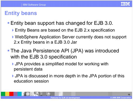
Entity bean support for EJB 3.0 has changed from previous versions of EJBs. While entity beans are still based on the EJB 2.x specification, EJB 3.0 has introduced a new method of data persistence called the Java persistence API, or JPA for short. In depth information on JPA tools is available in the Rational Application Developer V7.5 JPA development tools section of the IBM education assistant.
