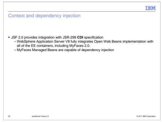
JSF 2.0 allows the use of the new JSR-299 Context and Dependency Injection specification for managed beans. This means a developer can replace the typical JSF managed bean with a CDI managed bean. For WebSphere Application Server V8, Open Web Beans was the CDI implementation used.
