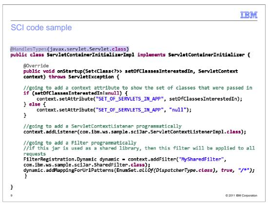
Here is a sample ServletContainerInitializer class file. Notice the HandlesTypes annotation which will cause the onStartup method to be called passing in all the javax.servlet.Servlet classes within the application along with the ServletContext. Also, notice that this ServletContainerInitializer programmatically adds a listener and filter.
