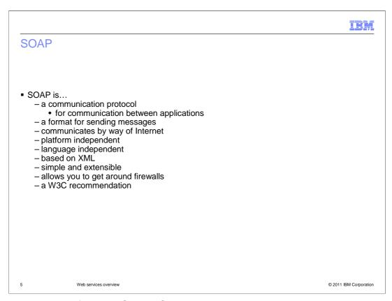
SOAP, originally defined as *Simple Object Access Protocol*, is a communication protocol specification for exchanging structured information in the implementation of web services in computer networks. It relies on XML as its message format, and typically relies on HTTP for message negotiation and transmission. SOAP provides a basic messaging framework upon which web services can be built.
