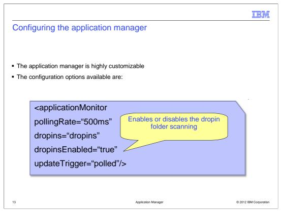
The "dropinsEnabled" element is a boolean to enable or disable adding and removing applications installed in the dropins directory. If you disable the dropins folder while the server is running any applications currently deployed from the dropins folder is removed from the server immediately.
