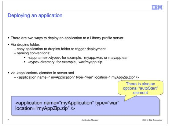
The other way to deploy an application is to add an application entry into the server.xml for the server. You can see an example server.xml entry at the bottom of the slide with four attributes:
