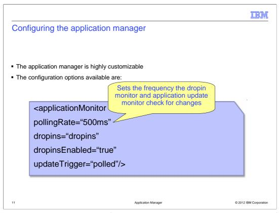
The "pollingRate" element sets the frequency between the dropin monitor looking for new applications or application removals, and how frequently the update monitor looks for changes to an application before updating it. The default value is "500ms" which is every half second.
