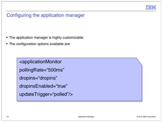
The application manager can be highly customized. All changes to the application manager occur under the "applicationMonitor" element in the server.xml.
