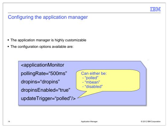
The "updateTrigger" element allows you to set how the server will detect updates to the applications. There are three options:
