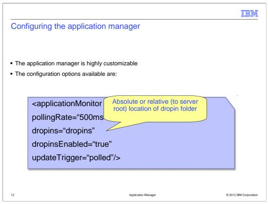
To move or rename the dropins folder use the dropins="" element where the content of the value for "dropins" is the location and name of the new dropins folder relative to the server's directory. If you change the dropins folders' location while the server is running any applications running from the old dropins folder is stopped.
