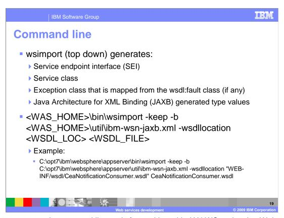
There are two main command line tools for working with JAX-WS to develop Web services. WSImport is a top down development tool that will create the necessary beans, service client, service endpoint interface, and wrappers from a provided WSDL file. The WSGen command will create a WSDL document and wrappers when needed from Java code with the proper Web service annotations.
