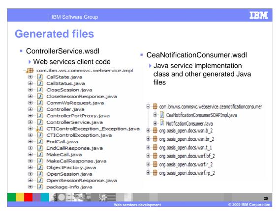
This picture shows the Web services client code that was generated from the ControllerService.wsdl file and the Java service implementation class and other oasis files that were generated from the CeaNotificationConsumer.wsdl file.
