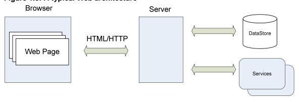
An Ajax design pattern allows the shifting of the balance of the user interface to the browser client. The creation of the viewable content can be shared between the browser
