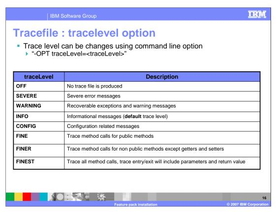
This slide is for reference; it lists the options to increase the log level for the installer.
