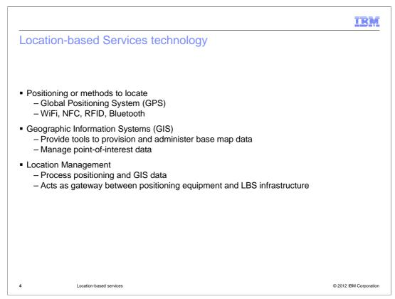
One of the most obvious technologies behind LBS is positioning or methods to locate. The most widely recognized system is the Global Positioning System (GPS), which is based on the concept of trilateration. There are however, other means of positioning in addition to GPS such as WiFi, NFC, RFID, and Bluetooth technologies used to match devices to nearby services based on their surroundings.
