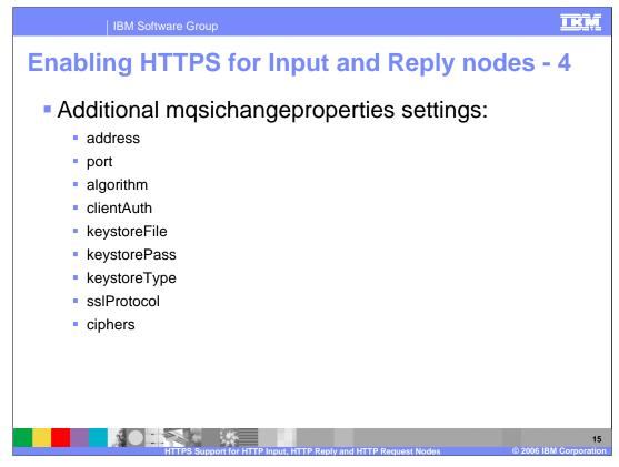
There are a number of other properties that can be set using mqsichangeproperties. Note that all of these values are simply passed straight through to the embedded Tomcat HTTP server. The Message Broker does not actually change these values in any way.
