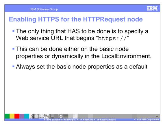
The HTTP or HTTPS address can be specified directly on the HTTPRequest node. Alternatively, it can be dynamically changed on a per connection basis.
