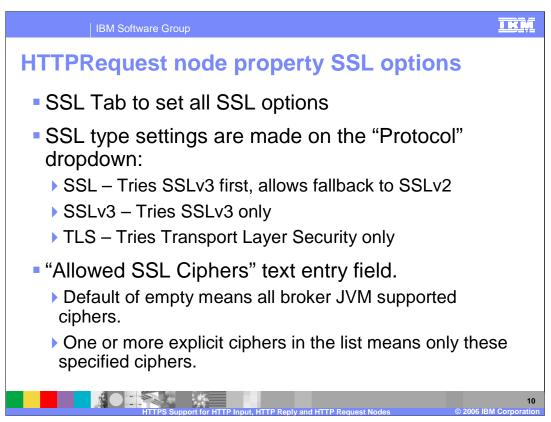
The first is an option called 'Protocol' which is presented as a drop-down combo box. This allows you to select which version of SSL to use. This can be SSL, SSLv3 or TLS. The default value is SSLv3.
