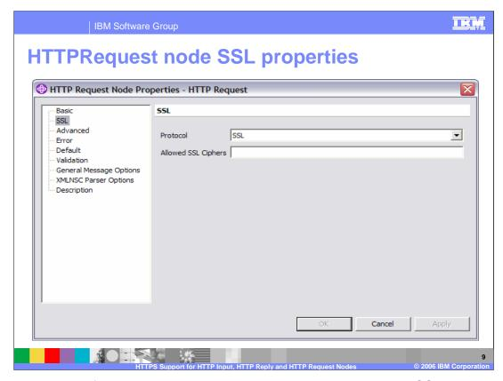
On the properties of the HTTPRequest node, there is a new tab called SSL. This tab is where all parameters related to SSL are located. There are two primary options on this tab.
