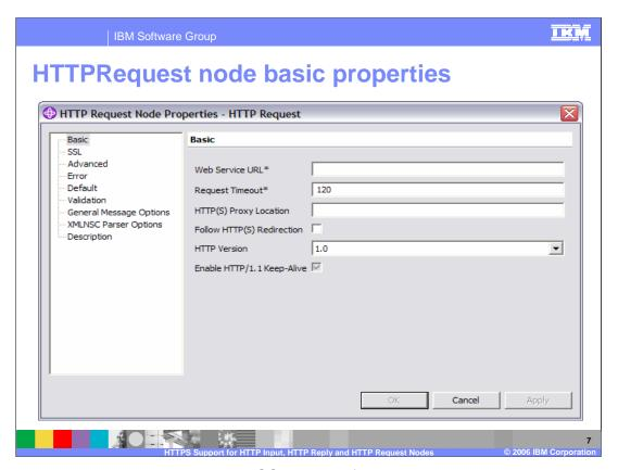
When using the HTTP Request node, SSL is specified simply by setting the URL to an identifier that begins 'HTTPS'. This is exactly the same process as using a web browser to connect over HTTPS. The HTTP or HTTPS address can be specified directly on the HTTPRequest node basic properties (Web service URL).
