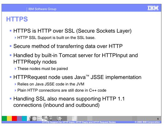
The support for HTTPS in the Version 6 broker simply means that the Secure Sockets Layer, or SSL, protocol is carried over a normal HTTP connection. It is the same support used for secure websites through a web browser.
