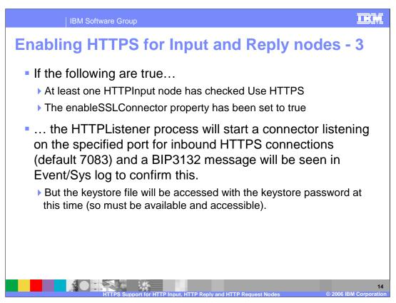
The HTTP Listener will start an SSL connector if the 'Use HTTPS' property on the HTTPInput node has been indicated and the 'enableSSLConnector' property has been set to true. The default port number for HTTPS connections is 7083, and when this is started a BIP3132 message will be seen in the event log or the system log which will say "Connector started for HTTPS".
