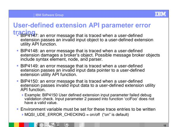
In Version 6, when a parameter error or object error is detected, a report of the error is now written to the broker trace log. Notice the new trace entries provided to report these errors, ranging from BIP4147 to BIP4150. These trace entries are controlled by MQSI UDE ERROR CHECKING environmental variable, which is set "on" by default.
