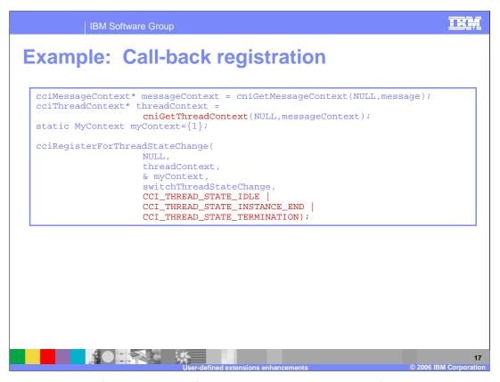
Here is an example of a registration for call-back, which monitors for thread idle, thread instance end, and thread termination.
