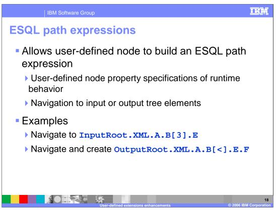
ESQL Path Expressions are allowed in WebSphere Message Broker Version 6. For example, you can create the path expression for a particular array element for input or output. Using path expressions allows the path to be more dynamic and can also reduce the number of function calls, especially if a target element is used a number of times and is deep within the tree structure.
