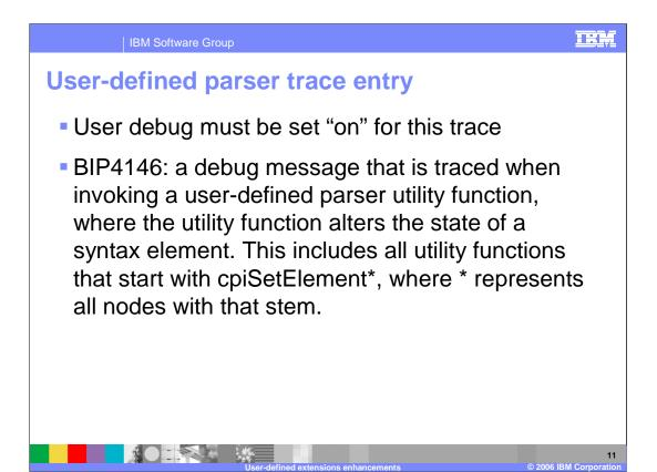
Trace entry BIP4146 is issued when a user-defined extension parser utility function alters the state of a syntax element. User debug tracing must be set "on" for this trace entry to be written.
