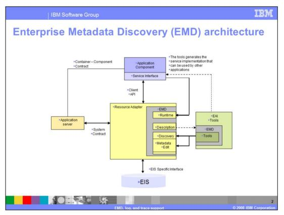
The slide shows an architectural view of Enterprise Metadata Discovery(EMD). The major portion of EMD is the tools contract, which specifies how the adapter can introspect the EIS and provide the necessary information to build a service. The EMD contract also has runtime contracts. The J2CA specification was designed before the introduction of SOA, so there are a few pieces necessary to bridge the gap between a "service" and a JCA connector. These are discussed later on in the presentation.
