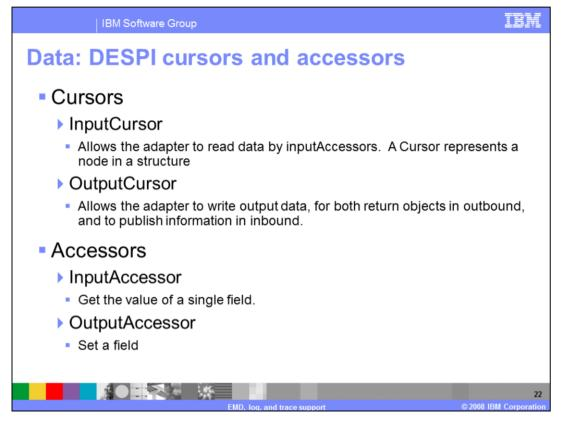
In Data Exchange Service Provider Interface (DESPI), data is accessed with cursors and accessors. A cursor represents a node in the structure. You can use the cursor APIs to traverse the structure, get the next object in a sequence of children, and so forth. An accessor represents a singe property or attribute. The accessor API allows you to manipulate a single piece of data, either getting or setting that data.
