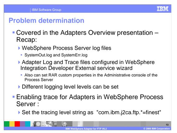
Listed here are the log files for WebSphere Process Server. The adapter logs the entries in the SystemOut.log and SystemErr.log files. You can also enable tracing for more detailed information. Note the trace string used to turn on tracing of the ftp adapter.
