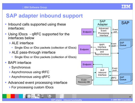
This diagram shows the high level flow and the components for the inbound events from SAP.
