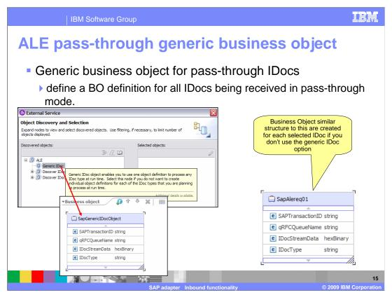
With V6.2 if you are going to use the ALE pass-through interface, you no longer need to generate a business object definition for each IDoc that is selected for import during configuration. Neither the control record nor the data record of the IDoc is parsed so there is no need for generation of business object specific for each IDoc. The business object will contain binary attribute to contain the IDoc content.
