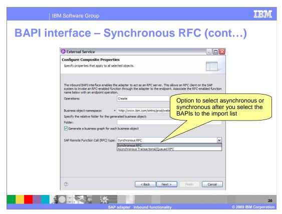
This slide shows the screen capture from the external service wizard where you can select between asynchronous or synchronous RFC support.
