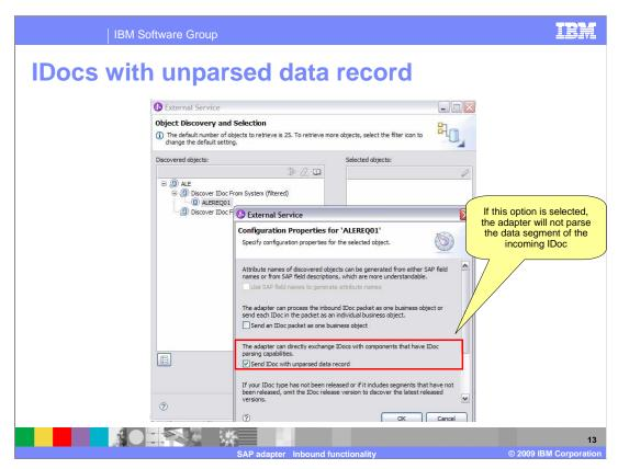
This slide shows the screen capture of the panel in external service wizard where you have the option to configure the adapter to not parse the data record of the incoming IDoc.
