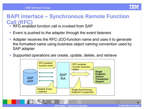
With V6.2, the adapter supports both synchronous and asynchronous RFC for events related to BAPI calls. So the Synchronous Callback Interface has been renamed to BAPI interface. The option of using synchronous or asynchronous is made after you select the BAPI calls you are interested in monitoring.
