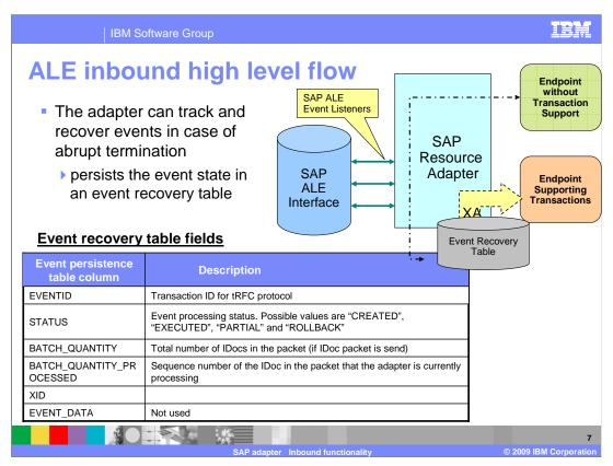
This diagram shows the components involved in end-to-end handling of the events. The SAP ALE event listeners listen for the events. The new event is pushed to the adapter, and the adapter stores it in the persistent event recovery table. The persistent table provides failure recovery to reprocess the events.
