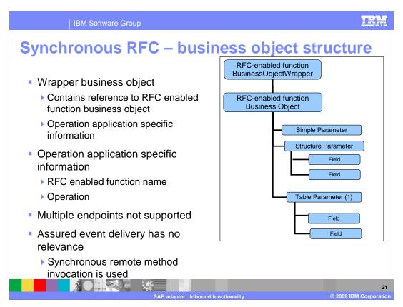
Adapter uses the wrapper business object application specific information to find the operation associated with received RFC-enabled function name .Once the operation is determined it is set as operation on business object before sending it to endpoint. Synchronous callback interface uses a synchronous remote method invocation. So, multiple endpoint support cannot be supported because each endpoint delivery requires synchronous response from endpoint.
