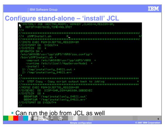
The zSMPInstall.sh script can also be run from JCL. This slide shows an example of running the shell script from JCL.
