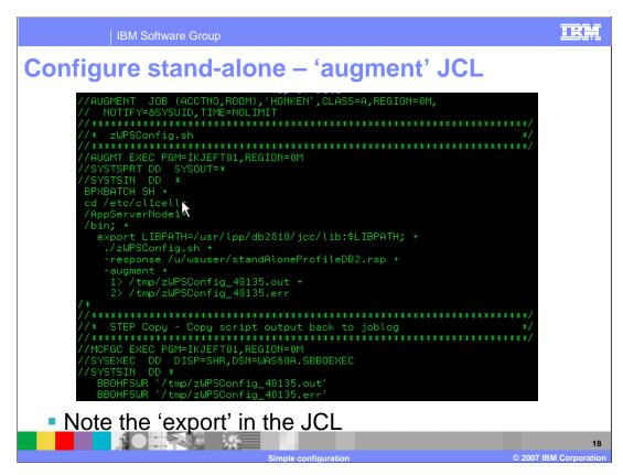
Again, here is an example of running the augment function using JCL. Do not forget to export the native Java common client LIBPATH if dbDelayConfig is set to 'false'.
