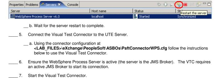
\_\_ a. From the start menu, select Programs > IBM WebSphere Business Integration Adapters > IBM WebSphere Business Integration Toolset > Visual Test Connector (VTC). This opens a command window in the background where the process runs and the Visual Test Connector Interface in the foreground. Do not close the command window as this will cause the VTC to exit.
