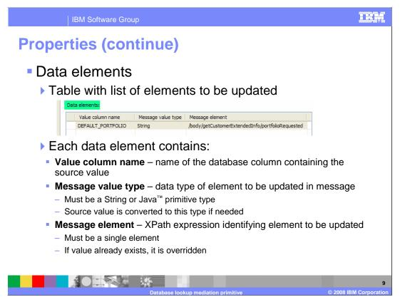
The final property for the database lookup primitive is the **Data elements** property. It is a table base property with three columns. Each row in the table identifies a specific element within the SMO that is updated using data obtained from the database.
