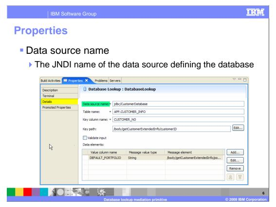
This screen capture shows the Details tab from the Properties view for a database lookup. The next several slides examine the various properties used to configure this primitive.
