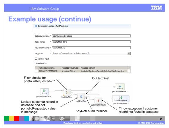
The top part of the slide shows the properties for the database lookup. The lookup is done on the CUSTOMER\_INFO table with a key column of CUSTOMER\_NO. The key value is obtained from the customerID element of the SMO message body. In the data elements table you can see that the value in the DEFAULT\_PORTFOLIO column is obtained and used to update the portfolioRequested element in the SMO body.
