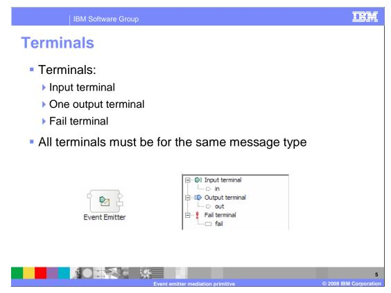
The event emitter primitive has one input terminal, one output terminal and a fail terminal. The output terminal must be for the same message type as the input terminal, because the event emitter primitive does not modify the message body. Shown here is an event emitter primitive with its terminals and the terminals as seen in the properties view.
