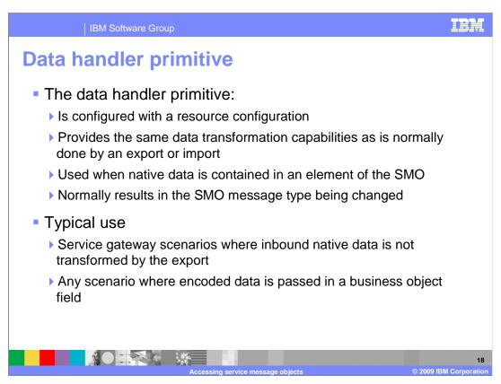
Similar to its use with imports and exports, the data handler primitive is configured with a resource configuration and provides the same data transformation capabilities of converting between native data and business object formats. The data handler converts between an SMO element containing native data and a section of the SMO representing a business object. Normally, this involves the changing of the SMO body and thus changing the message type of the SMO.
