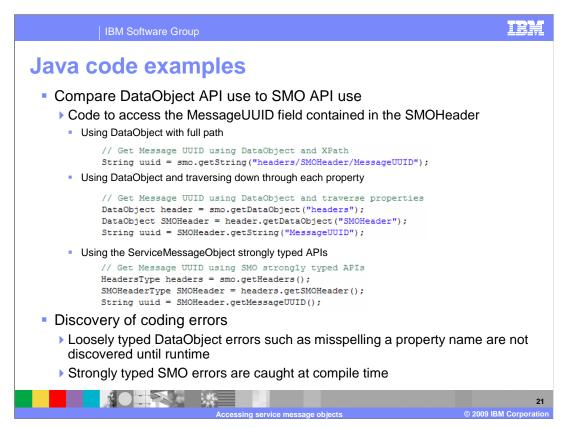
This slide compares the use of the DataObject APIs to the ServiceMessageObject APIs by using three examples that do the same thing. They each access the MessageUUID field that is in the SMOHeader.
