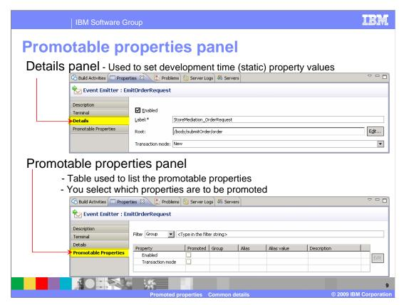
In the properties view for a mediation primitive, two of the panels provided are the details panel and the promotable properties panel.
