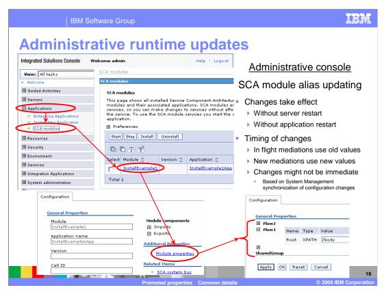
Screen captures from the administrative console are shown here to illustrate how to display and update aliases for an SCA module in an installed application.
