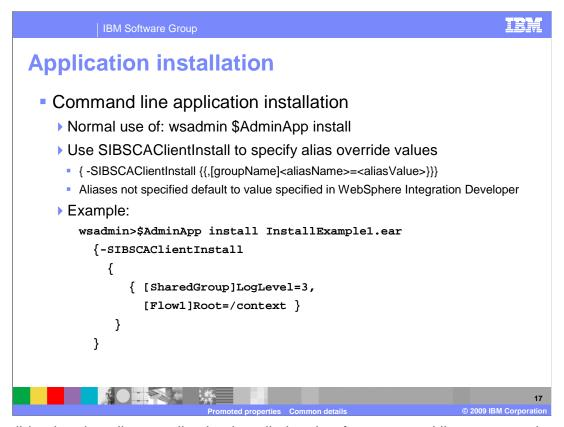
This slide also describes application installation, but for command line usage rather than through the administrative console. It makes use of the wsadmin \$AdminApp install command with the SIBSCAClientInstall option. The syntax for the command and an example are shown in the slide. Any aliases not specified using this option default to the value given to the alias in the WebSphere Integration Developer.
