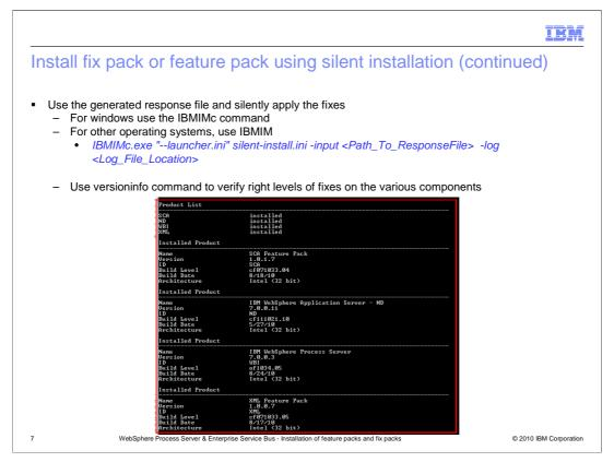
Once you have the response file generated, you can now use the Install manager to silently install the feature pack or fix pack. You can use the IBMIMc command for windows operating system and IBMIM for other OS. An example of the usage is shown here in the slide.
