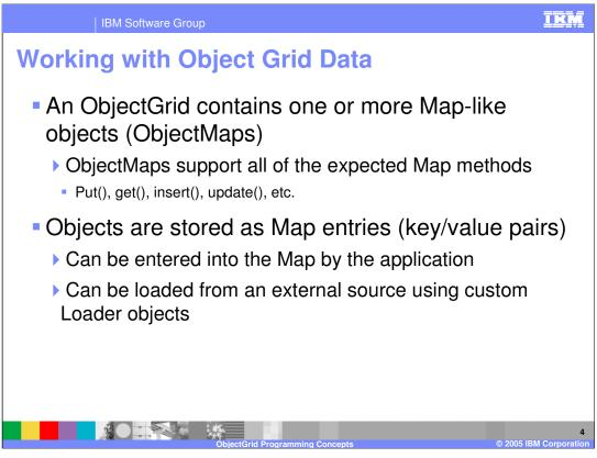
Java<sup>™</sup> Objects are stored in an ObjectGrid using key-value pairs within Map objects called ObjectMaps. Data can be put into and retrieved from an ObjectMap using all of the usual Map-like methods, within the scope of a transaction. The Map can be solely populated by the application, or it can be loaded from a back-end store by implementing a custom cache loader.
