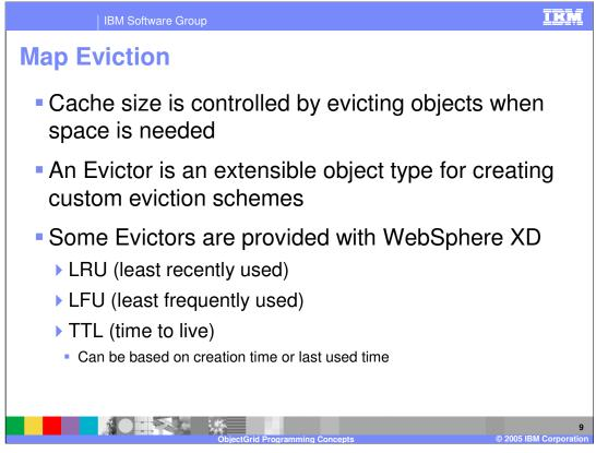
Cache size control is also customizable. WebSphere XD provides Evictor classes that can remove objects from the cache using least-frequently used or least-recently used policies, when the cache reaches a certain size, and also a time-to-live based evictor for invalidating entries that have existed for longer than a set period of time. You can also write your own evictor class, to manage the cache size based on custom criteria.
