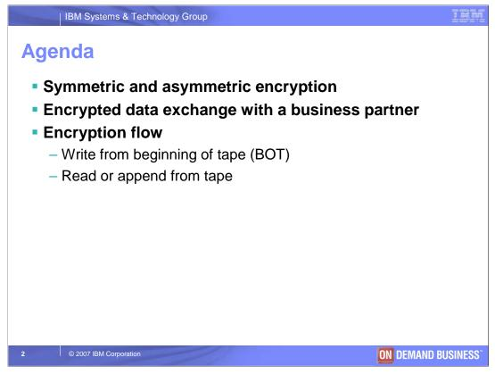
This module will start by going over symmetric and asymmetric encryption terminology with a discussion of how each plays a role in the 3592 Model E05 tape encryption support. Then it will walk you through a detailed example showing a business partner data exchange and what each company would have in its key store. You will see the steps involved in a write from the beginning of tape, followed by the steps involved in a tape read or an append.
