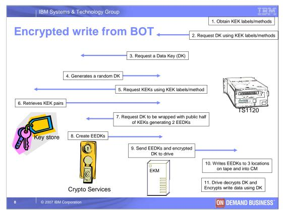
This is a high level view of some of the steps involved in an encrypted write. In this case the write is from the beginning-of-tape (BOT) and shows the roles that the tape drive, the EKM, crypto services and the key store play in the overall solution.
