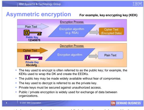
The asymmetric key also referred to as a public/private key pair is used in the tape encryption solution to encrypt "wrap" and decrypt the data key. The public key is used to encrypt the data key and the private key is used to decrypt the data key. The encrypted data key is stored on the tape cartridge in a structure referred to as the externally encrypted data key (EEDK).
