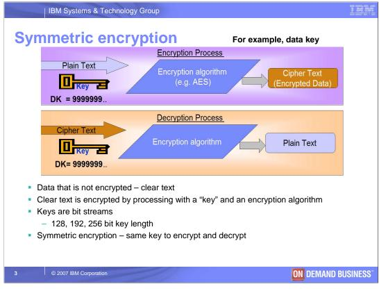
The symmetric key also referred to as the "data key" in the tape encryption solution is used by the tape drive to encrypt and decrypt the data on the tape cartridge.
