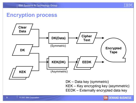
This picture shows the role that the data key has in encrypting the data stored on the tape cartridge and the role that the key encrypting key plays in encrypting the data key. When the encryption process completes not only is encrypted data placed on the tape cartridge, but along with the data, the drive also stores the encrypted data key.
