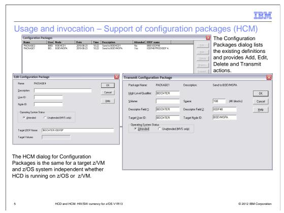
In the Create Configuration Package Dialog you have to specify at least the target IODF name. HCM accepts both MVS and VM IODF names because it may be determined later whether the IODF is sent to a z/VM system or to a (attended or unattended) z/OS system. If a file type of PRODIODF is given, the syntax is validated against VM IODF name convention, otherwise against MVS IODF name rules.
