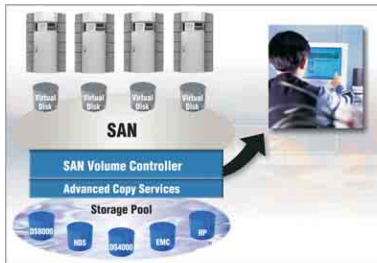
Figure 1 - SVC helps combine capacity from different storage systems, helps provide common copy functions and enable data movement without server disruption, and is designed to support management of diverse storage from a single point.
