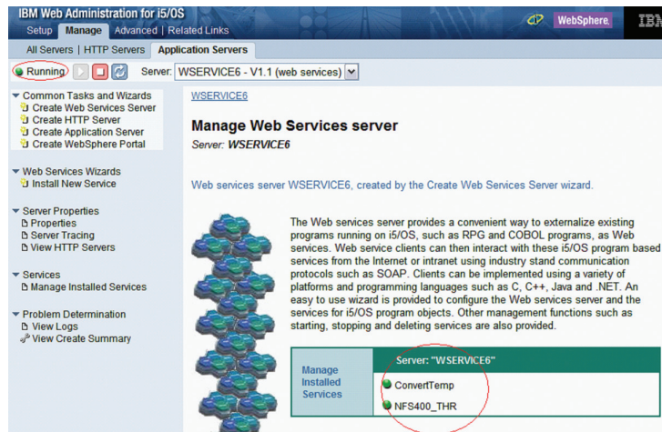
Figure 2. When created, the server and the deployed service are started.
