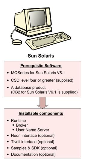
Figure 1. Planning for installation
