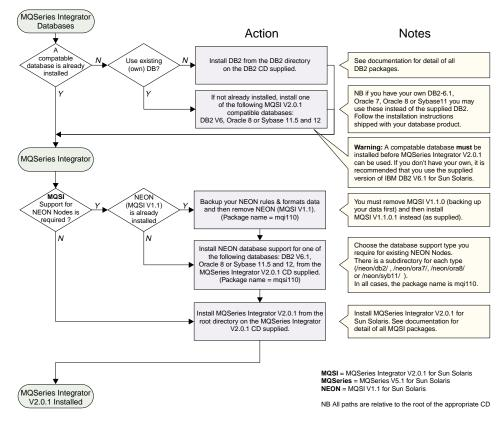
Figure 5. Installation of MQSeries Integrator for Sun Solaris, part 2
