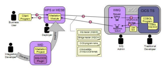
The plug-in provides mediation primitives that allow you to specify the MQ message headers options for MQMD and MQCIH and also provides header binding class for constructing a MQ message that can be handled by the MQ-CICS bridge. Instead of taking days or weeks to develop integration code to access your CICS applications, it should only take about an hour or even less with the plug-in.
