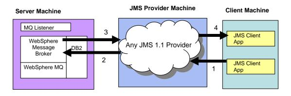
The numbered arrows indicate the sequence of processing:
