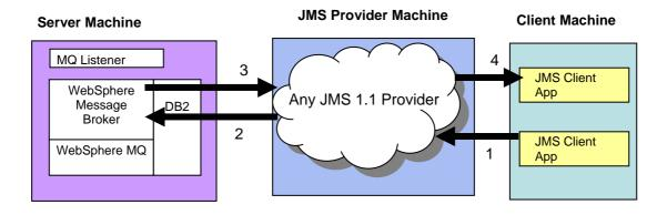
The numbered arrows indicate the sequence of processing:
