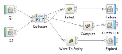
The two MQ Input nodes all propagate messages to the collector node. In
