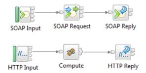
The SOAPRequest node is used in a message flow that calls a web service synchronously. This means the node sends a Web Service request and waits for the associated web service response to be received before the message flow continues.
