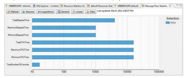
The overhead of using this facility was measured when running a ESQL Transform test using the XMLNSC parser processing a 2KB input message. The processing overhead was measured at 6%. This is a very small overhead for the quality of the data collected.
