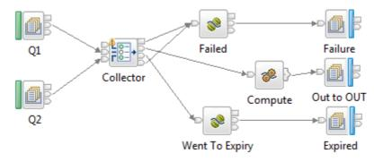
The two MQ Input nodes each propagate messages to the collector node. In the collector node a collection is defined as being 1 input message
