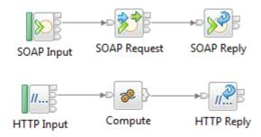
The SOAPRequest node is used in a message flow that calls a web service synchronously. This means the node sends a Web Service request and waits for the associated web service response to be received before the message flow continues.
