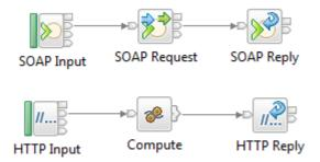
The SOAPRequest node is used in a message flow to invoke a web service synchronously. A response must be received from the web service before the message flow continues.
