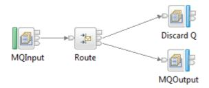
The MQ Input node is set to use the XMLNSC domain. Within the Route node the first element of the message is queried and the message routed based on this value. The lookup result is always set to be true and thus the message is propagated to the MQ Output node.
