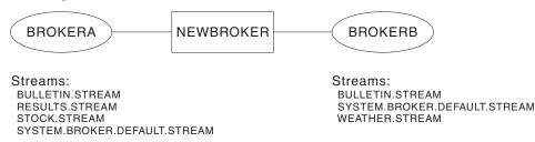
The default stream queue SYSTEM.BROKER.DEFAULT.STREAM is always supported by every broker in an WebSphere MQ Publish/Subscribe network, and must be defined at every WebSphere Event Broker broker in a heterogeneous network. At each broker, you must define and deploy a message flow to service this queue.
