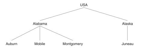
Each character string in the figure represents a node in the topic tree. A complete topic name is created by aggregating nodes from one or more levels in the topic tree. Levels are separated by the "/" character. The format of a fully specified topic name is: "root/level2/level3".
