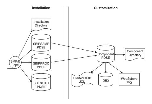
To perform the customization, update and submit the required JCL. All necessary JCL is supplied to create the runtime environments of your broker, Configuration Manager, and User Name Server. You start the broker, Configuration Manager, or User Name Server using one of the supplied JCL files, which is run as a started task.
