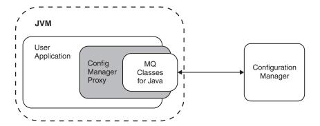
The CMP application can be on the same physical machine as the Configuration Manager, connected by a JNI (Java Native Interface) connection to the queue manager using the WebSphere MQ Java Bindings transport, or distributed over a TCP/IP network, and connected to the queue manager by a WebSphere MQ SVRCONN channel using the WebSphere MQ Java Client transport.
