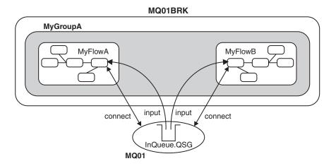
This example demonstrates that the serialization token is restricted within a single execution group running on a broker::
