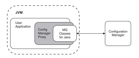
The CMP application can be on the same physical machine as the Configuration Manager, connected by a JNI (Java Native Interface) connection to the queue manager using the WebSphere MQ Java Bindings transport, or distributed over a TCP/IP network, and connected to the queue manager by a WebSphere MQ SVRCONN channel using the WebSphere MQ Java Client transport.
