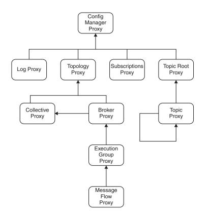
Using the ConnectToConfigManager example as a starting point, the following program traverses the administered object hierarchy to discover the run state of a deployed message flow. Note that the program assumes that message flow MF1 is deployed to EG1 on broker B1, although it is possible to substitute these values in the code for any that are valid in the domain.
