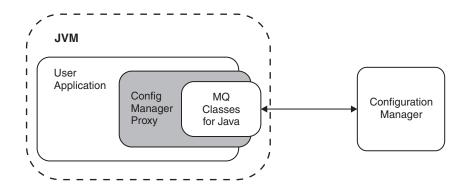
The CMP application can be on the same physical machine as the Configuration Manager, connected by a JNI (Java Native Interface) connection to the queue manager using the WebSphere MQ Java Bindings transport, or distributed over a TCP/IP network, and connected to the queue manager by a WebSphere MQ SVRCONN channel using the WebSphere MQ Java Client transport.
