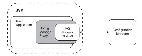
The CMP application can be on the same physical machine as the Configuration Manager, connected by a JNI (Java Native Interface) connection to the queue manager using the WebSphere MQ Java Bindings transport. Alternatively, it can be distributed over a TCP/IP network, and connected to the queue manager by a WebSphere MQ SVRCONN channel using the WebSphere MQ Java Client transport.
