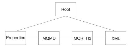
These elements at the first generation are often referred to as folders, in which syntax elements that represent message headers and message content data are stored. In this example, the first child of root is the Properties folder. The next sibling of Properties is the folder for the MQMD header. The next sibling is the folder for the MQRFH2 header. The last folder represents the message content, which (in this example) is an XML message.
