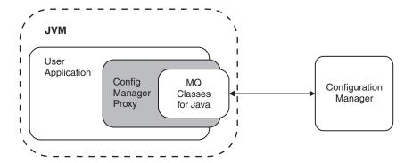
The CMP application can be on the same physical machine as the Configuration Manager (JNI to the queue manager using the WebSphere MQ Java Bindings transport) or distributed over a TCP/IP network (a WebSphere MQ SVRCONN channel using the WebSphere MQ Java Client transport).
