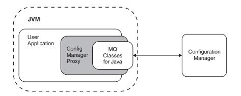
The CMP application can be on the same physical machine as the Configuration Manager (JNI to the queue manager using the WebSphere MQ Java Bindings transport) or distributed over a TCP/IP network (a WebSphere MQ SVRCONN channel using the WebSphere MQ Java Client transport).
