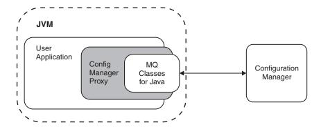
The CMP application can be on the same physical machine as the Configuration Manager, connected by a JNI (Java Native Interface) connection to the queue manager using the WebSphere MQ Java Bindings transport. Alternatively, it can be distributed over a TCP/IP network, and connected to the queue manager by a WebSphere MQ SVRCONN channel using the WebSphere MQ Java Client transport.
