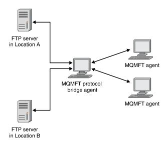
The diagram shows two FTP servers, at different locations. The FTP servers are being used to exchange files with the Managed File Transfer agents. The protocol bridge agent is between the FTP servers and the rest of the MFT network, and is configured to communicate with both FTP servers.
