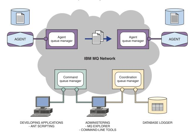
The diagram shows a simple Managed File Transfer topology. There are two agents, each connect to their own agent queue manager in an IBM® MQ network. A file is transferred from the agent on the one side of the diagram, through the IBM MQ network, to the agent on the other side of the diagram. Also in the
