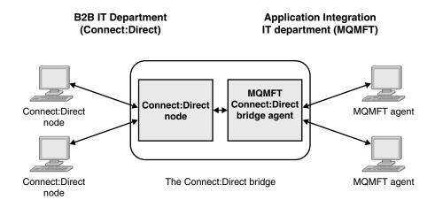
The diagram shows an MFT Connect:Direct bridge between two departments, the B2B IT department and the Application Integration IT department. The B2B IT department uses Connect:Direct to transfer files to and from the company's business partners. The Application Integration IT department uses IBM MQ as its messaging infrastructure and so has recently chosen Managed File Transfer as its file transfer solution.
