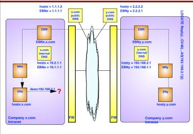
➤ The control vectors representing an EE connection network carry the IP address of the node that owns the vectors.
