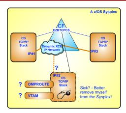
The assumption is that if a TCP/IP stack determines it can no longer perform its Sysplex functions correctly, it is better for it to leave the TCP/IP XCF group and by doing so, signal the other TCP/IP stacks in the Sysplex that they are to initiate whatever recovery actions have been defined, such as moving dynamic VIPA addresses or removing application instances from distributed application groups.
