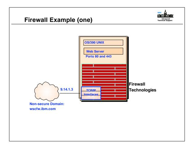
• OS/390 system, running a web server , connected to the Internet. A firewall is setup on this host to ensure that only traffic destined for the Web server are allowed in. All other data is denied access.
