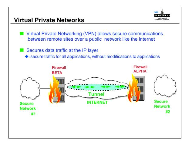
• Illustrated is a tunnel between two firewall hosts across the Internet. The two secure networks are in effect combined into a Virtual Private Network and it allows secure communications between the two hosts.
